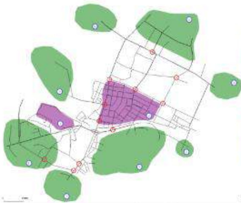
Zones with starting and ending points for traffic movements and marked traffic lights
